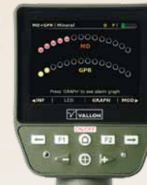
Different graphical representation of alarms, either by LEDs or by charts.
