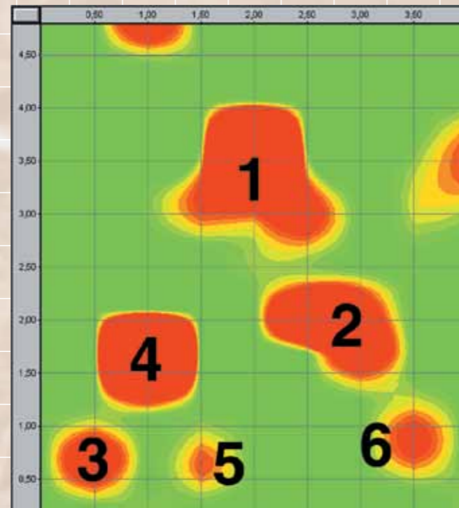
no. 1 = 50 kg aerial bomb at 1.7 m depth no. 2 = 75 mm tank grenade at 1.2 m depth
