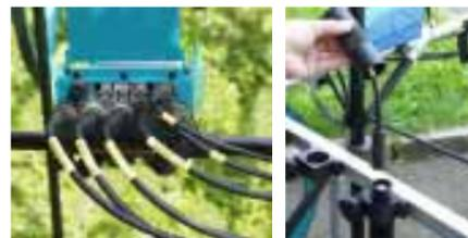
The Field Computer VFC1 is very compact and can be used under all weather conditions. Up to 4 detectors and a positioning system can be connected.
