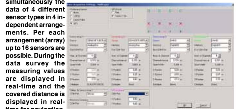
simultaneously the data of 4 different sensor types in 4 independent arrangements. Per each arrangement (array) up to 16 sensors are possible. During the data survey the measuring values are displayed in real-time and the covered distance is displayed in real-time for navigation.
