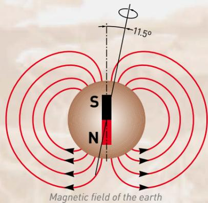
The magnetic field of the earth is homogeneous with regards to the field strength and the direction of the field strength. If a ferromagnetic object is brought into this homogeneous field, the own field of the object is superposing the local homogeneous magnetic field of the earth.
