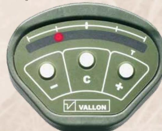
According to the polarity of the magnetic inhomogeneity, the LED-signal is shifted to the left or to the right side. The position of the LED is proportional to the strength of the detection signal.
