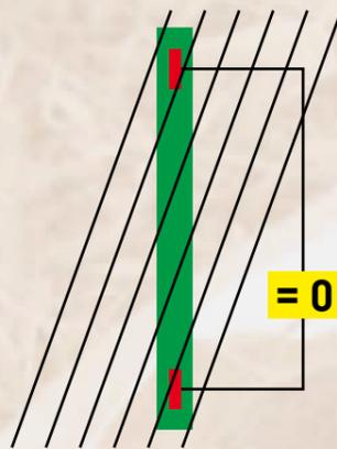
The VXC1 is a differential magnetometer, i.e. two sensors are arranged in geometrically true alignment with a distance of 300 mm and are connected in a way that they measure the value zero in a homogeneous field.
