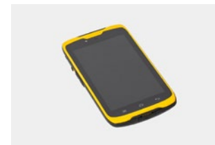
VFC4 – Small Field Computer for EVA4mobile® Art.-Nr. 2005350000
